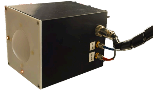
Teflon dielectric lens to enhance the radar spatial resolution and sensitivity
